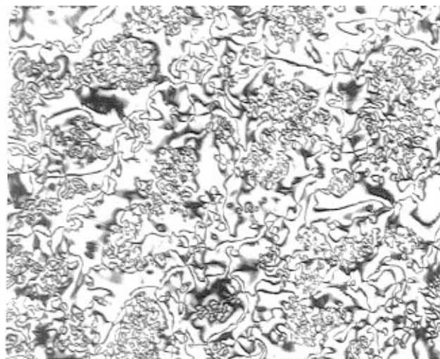
Figure 2. Polarizing optical micrograph of the 50/50 blend of samples 1 and 2 at 80 °C. Magnification: 170 \times .
